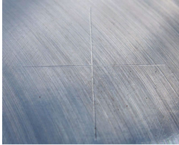
Figure 4.3: Alignment lines for a target strain gauge rosette (photo courtesy of Stresscraft Ltd.).
