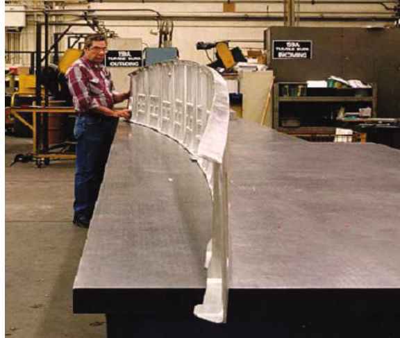
Figure 1.14: C-17 cargo ramp warped by the release of residual stresses within the material machined away during manufacture (photo courtesy of D. Bowden, Boeing Company).
