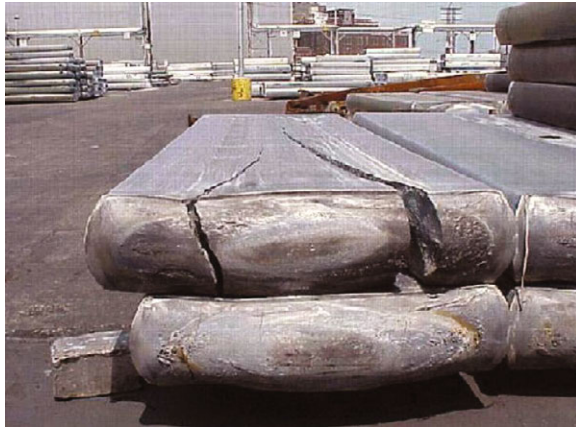
Figure 1.6: Cracking of a cast aluminum ingot due to excessive residual stresses (photo courtesy of Mark Newborn, Alcoa).
