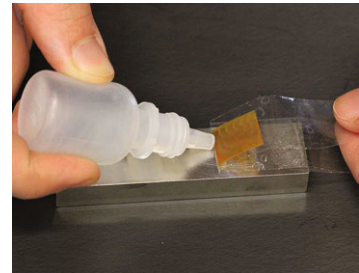
(f) Application of adhesive
