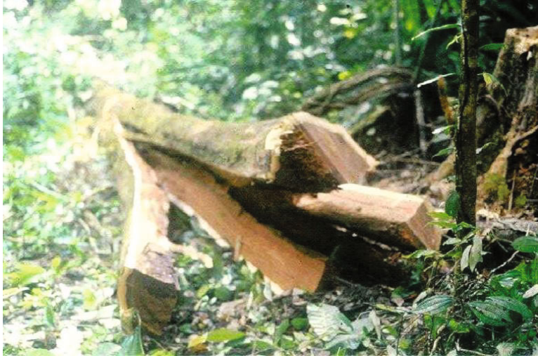
Figure 1.13: Growth stresses in a eucalyptus tree caused the trunk to split open after felling (photo courtesy of Wood Machining Institute).
